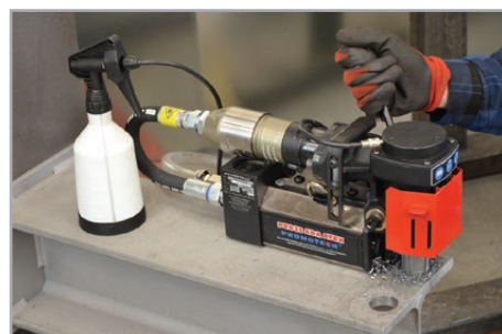
Through spindle cooling system
